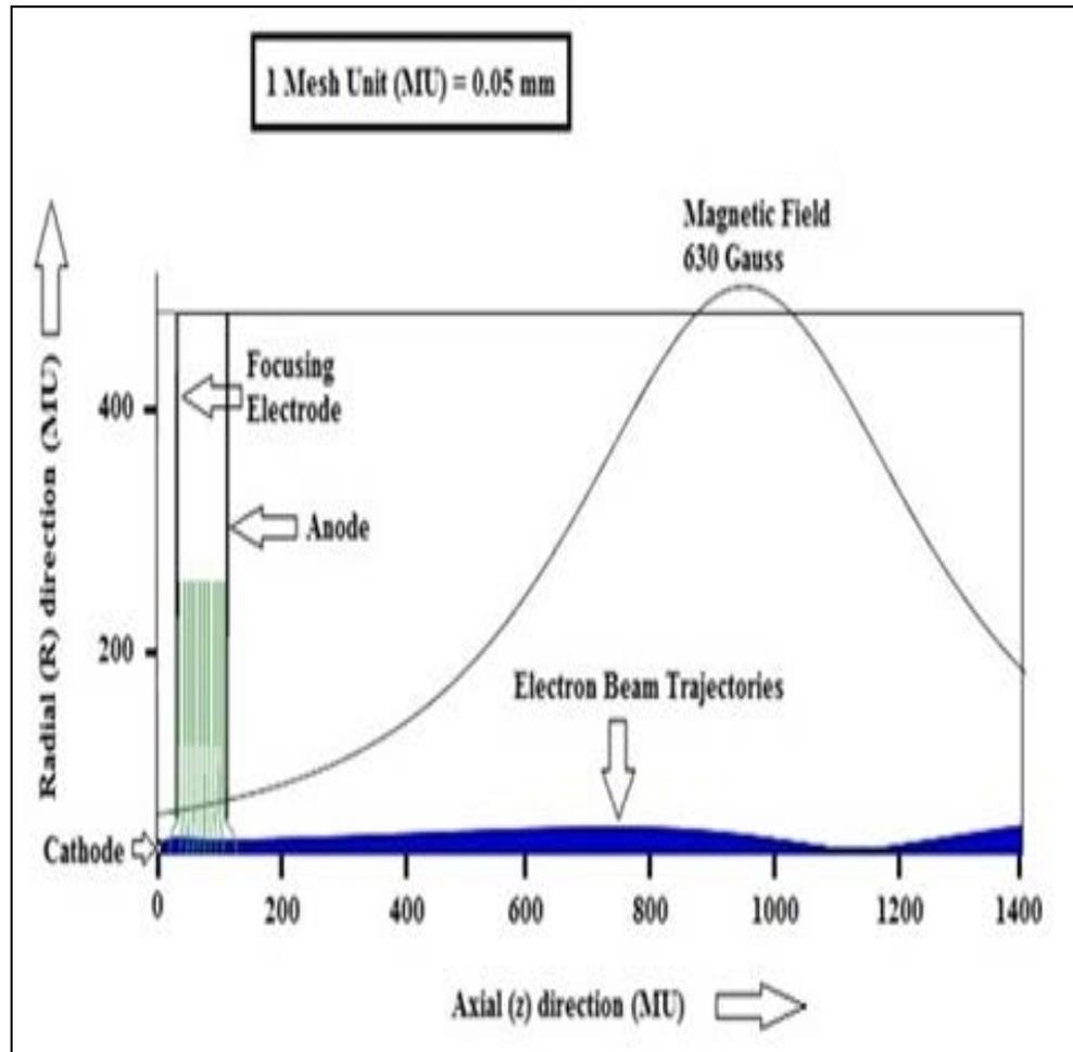
Two dimensional (2-D) Plot of beam trajectories.
