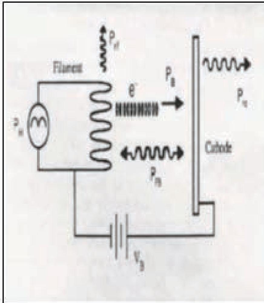
Schematic view of an indirectly heated cathode model
