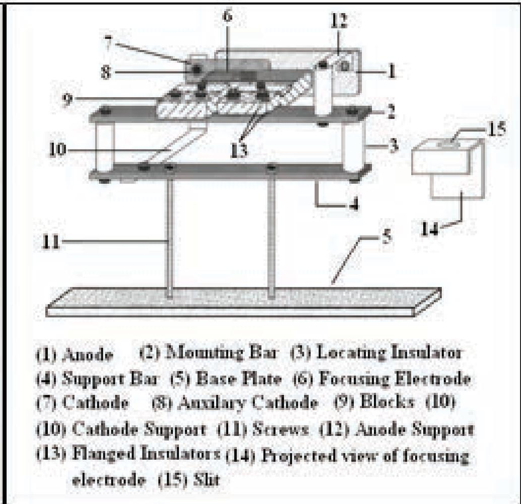
Schematic view of the strip source electron gun
