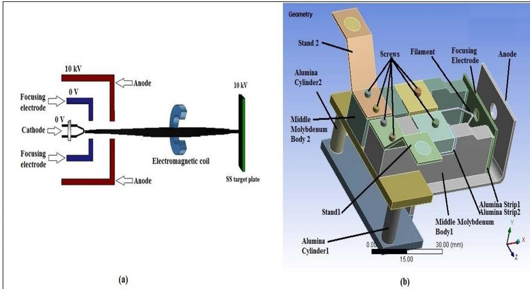
(a) Two dimensional schematic view of the gun with electromagnetic coil and target, and (b) Three dimensional model of the gun.
