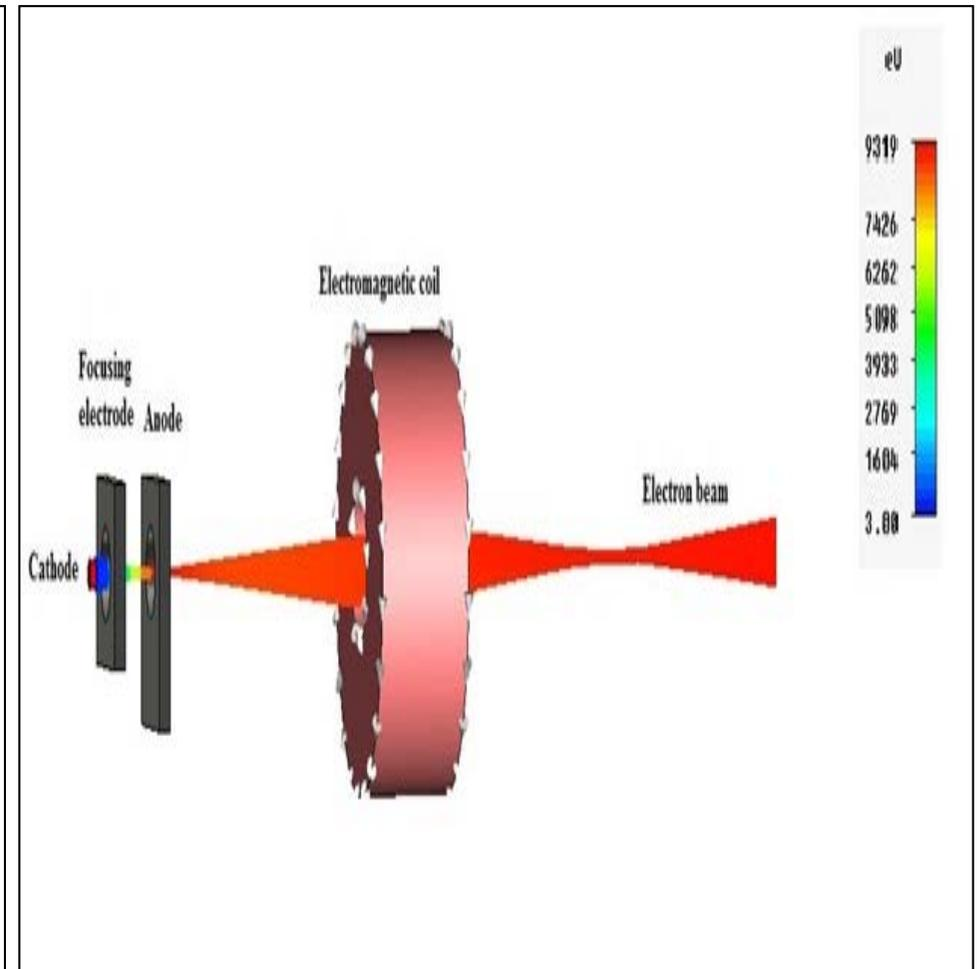
Three dimensional (3-D) schematic of the gun and its convergence with the coil.
