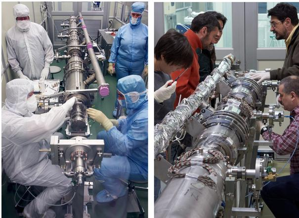
Figure 5: Assembly work of the cryomodules in progress.
