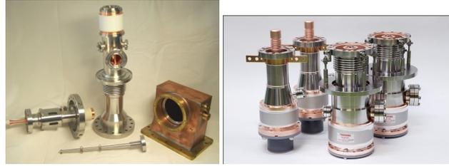
Figure 2: TTF-III (left) and STF-II (right) couplers.
