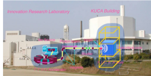
Figure 1: Schematic layout of ADSR experiment with 150MeV proton FFAG accelerator complex at KURRI.
