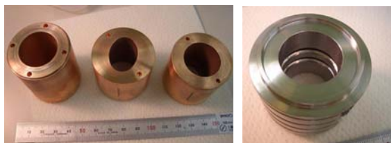
Fig. 8 Parts for the present load. Left: elliptical polarizer and right: lossy load cell.
