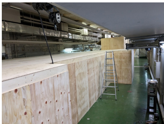
Figure 3: L-band linac covered with wooden boards.
