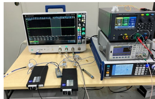
Figure 3: a) Block diagram and b) photo of the simplified baseband IQ detection system.
