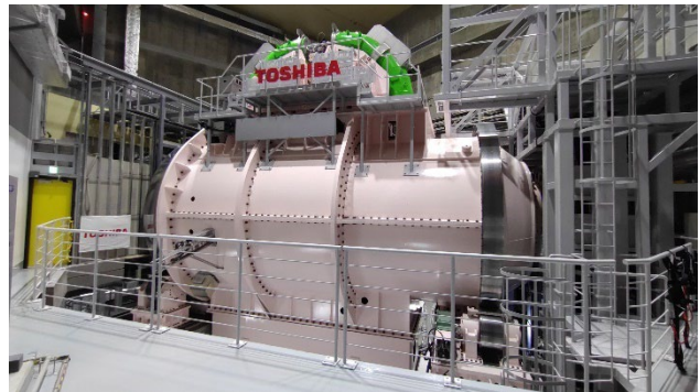
Figure 1: Rotating gantry for carbon ion radiotherapy with combined function superconducting magnets developed by Toshiba Energy Systems and Solutions installed at Yamagata University.
