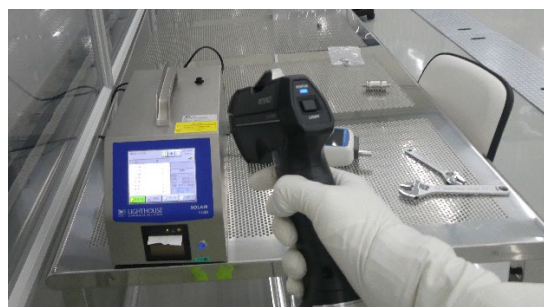
Figure 9: Photo of particle measurement at ISO class 4 (class 10).
