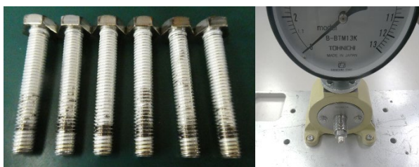
Figure 2: (Left) Discarded Teflon-coated silver-plated bolt (SUS316L), (Right) View of axial force measurement with washers in position.
