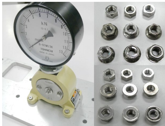
Figure 6: (Left) View of axial force measurement. (Right up) Front side of each nut. (Right bottom) Backside of each nut.
