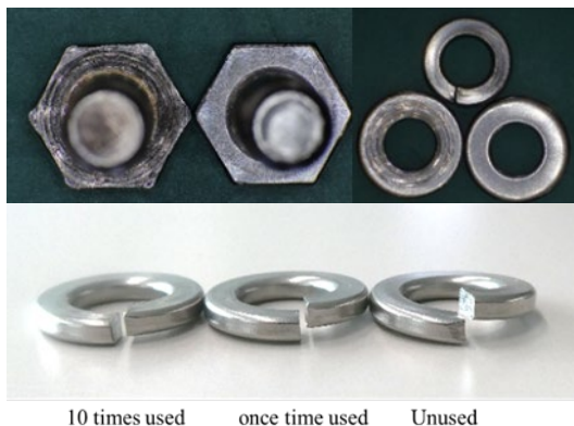
Figure 3: (Upper Left) From the left used bolt, new bolt. (Upper Right) Upper is spring washer, from bottom the left used washer, new washer. (Bottom) From left: 10 times used spring washer, once time used spring washer, new spring washer.
