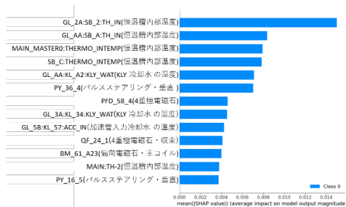
Figure 10: Critical parameters for the SY3 beam loss predicted by SHAP. The top 13 out of 1499 parameters are shown.
