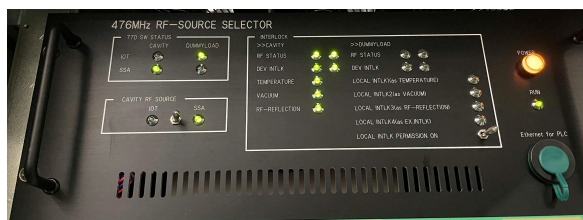
Figure 5: Photo of the RF source selector.
