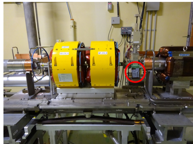
Figure 7: Irradiation setup at LINAC. The red circle indicates the light-shielding bag containing the films and dosimeters.
