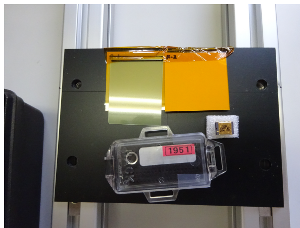
Figure 2: A jig for irradiating films and dosimeters between acrylic planes.
