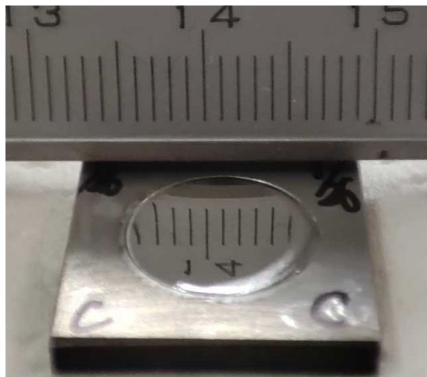
Figure 3: EP-treated Nb substrate by dynamic polarization.
