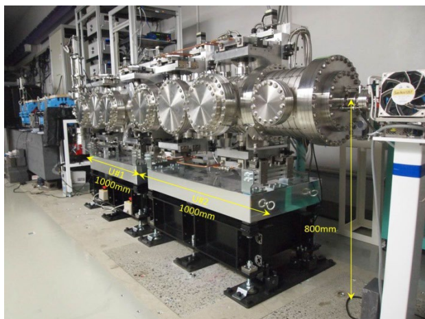
Figure 7: Photograph of the JST-MIRAI XUV-FEL undulator 2 m long. It is composed of 2 segment undulators (U#1 and U#2), 1 m long each. The gap of each segment can be changed independently.
