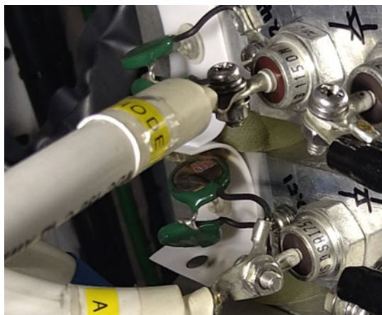
Figure 8: Broken varistors and diodes of droop compensation circuit.
