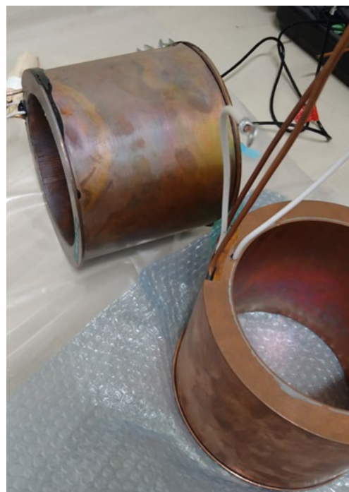
Figure 10: Black resin material can be seen seeping through the gap in the case of the damaged coil on the far side. The coil in the front side is a new one.
