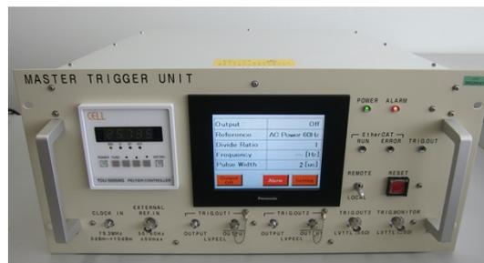
Figure 3: Photo of the Master Trigger Unit.
