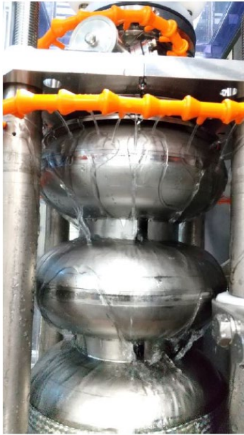
Figure 4: Cavity cooling with pure water.
