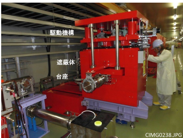
Figure 1: MR beam collimator. (At the time of Col-E main part line out).
