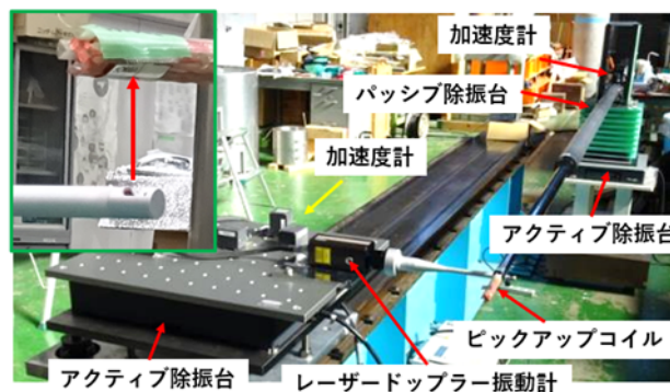
Figure 9: Set-up configuration of vibration measurement system with laser doppler vibrometer.
