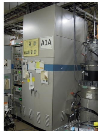
Figure 5: The small modulator using the highly precise inverter PS (left) and the klystron (right).
