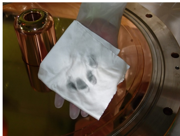
Figure 3: Wiping cloth after wiping inner surface of the end plate of S05B.
