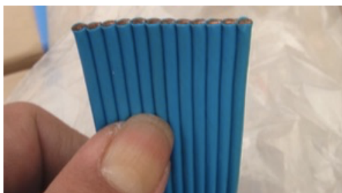
Figure 8: 12-turn flat cable used for demagnetization coils.
