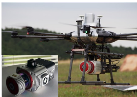
Figure 6: UAV lidar system (Asia Air Survey Co., Ltd.).
