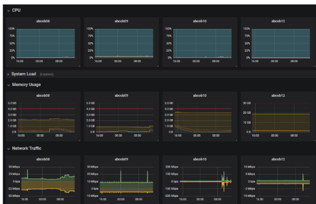
Figure 1: Grafana dashboard for computer performance monitoring. Each metrics is collected by SNMP.
