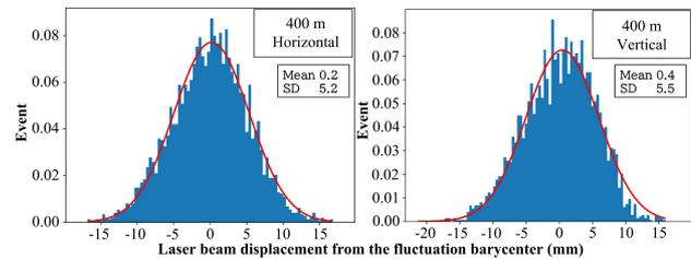
Figure 3: Laser stability after 400 meters of transmission with spherical mirrors.
