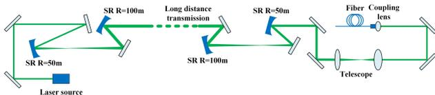
Figure 2: Experimental layout of the 400 m long-distance transmission experiment with spherical mirrors.
