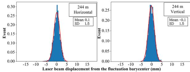
Figure 6: Laser stability after 244 meters of transmission in the KEKB tunnel.
