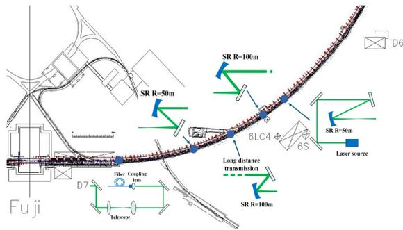
Figure 5: Experimental layout in the KEKB tunnel.
