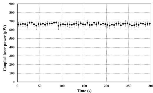
Figure 7: Coupled laser power after 244 m of transmission in the KEKB tunnel.
