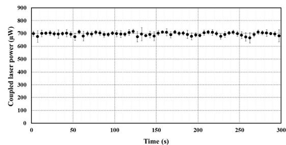
Figure 4: Coupled laser power after 400 m of transmission.
