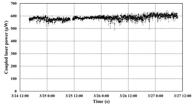
Figure 8: The 64-hour laser power history was recorded in the ground power supply building.
