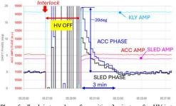
Phase feedback is turned on after waiting 3 minutes after HV is turned on. Beam injection to the rings also starts 3 minutes after HV is turned on.
