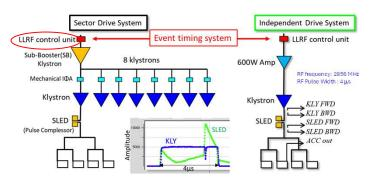
LLRF unit receives beam mode information and RF setting phase directly from the event timing system via optical fiber for each pulse and generates RF pulses.
