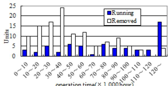
Figure 1: Klystron age profile as of March 2024.
