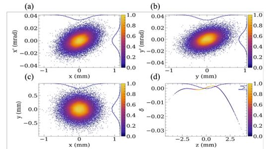
Figure 3: Initial beam distribution on the (a)  $x-x'$ , (b)  $y-y'$ , (c)  $x-y$ , and (d)  $z-\delta$  planes, with normalized histograms in dark-blue before the 7-GeV electron beam transport. The color code indicates the density of the beam.
