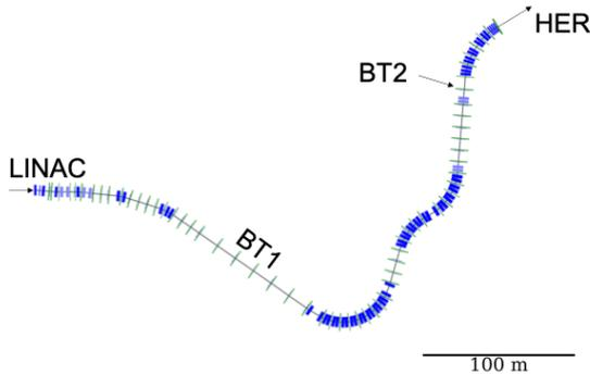
Figure 1: 7-GeV electron beam transport between the SuperKEKB high-energy ring (HER) and the LINAC. It comprises two achromatic sections of BT1 and BT2. The bending and quadrupole magnets are indicated in blue and green, respectively.
