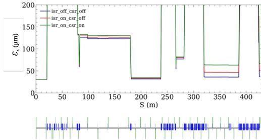
Figure 9: Evolution of the normalized horizontal emittances. The normalized horizontal emittances at the injection point 1) without ISR and CSR, 2) with ISR, and 3) with ISR and CSR are 38, 52, and 66  $\mu\text{m}$ , respectively.
