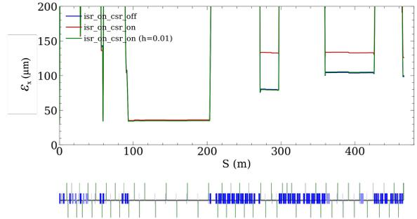
Figure 10: Evolution of the normalized horizontal emittances with narrower beam duct. The normalized horizontal emittances at the injection point 1) with ISR (blue), 2) with ISR and CSR (red), and 3) with ISR and CSR and a duct height of 10 mm (green) are 99, 126, and 100  $\mu\text{m}$ , respectively.
