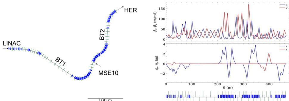
Figure 1: 7-GeV electron beam transport between the SuperKEKB high-energy ring (HER) and the LINAC.
