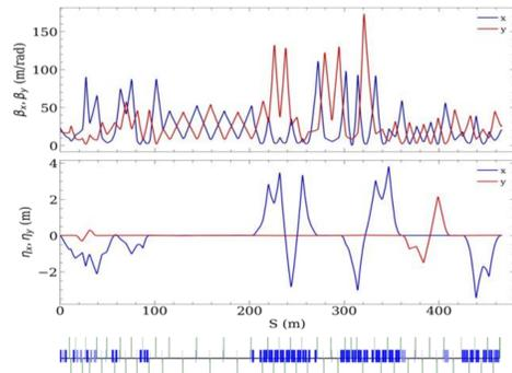
Figure 2: The nominal optics of the electron beam transport.
