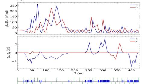
Figure 8: An optics for the new electron beam transport.
