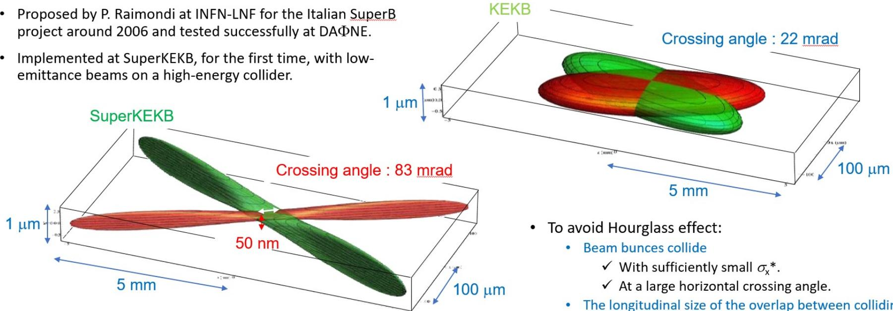
$$\left\{ \begin{aligned} L &\approx \frac{\gamma_{\pm}}{2e r_e} \left( \frac{I_{\pm} \xi_{y\pm}}{\beta_{y\pm}^*} \right) \\ \xi_{y\pm} &\approx (r_e N_{\mp} / 2\pi \gamma_{\pm} \sigma_{x,eff}^*) \sqrt{\beta_y^* / \epsilon_y} \text{ constant} \end{aligned} \right. \Rightarrow \left\{ \begin{aligned} L &\propto \frac{I_{\pm}}{\beta_{y\pm}^*} \\ L_{sp} &\equiv \frac{L}{n_b I_b - I_{b+}} \propto \frac{1}{\beta_{y\pm}^*} \end{aligned} \right.$$
