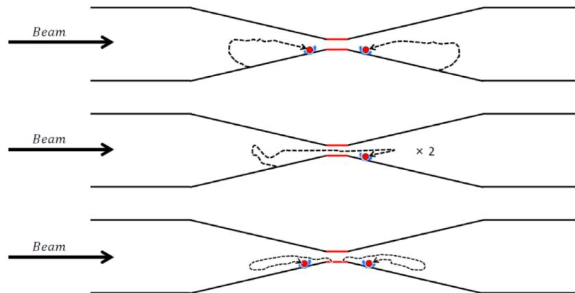
When a tiny particle is heated up by the beam-induced field and then touches some metal surface, it generates plasma and causes vacuum arc, which could interact with beam particles.
