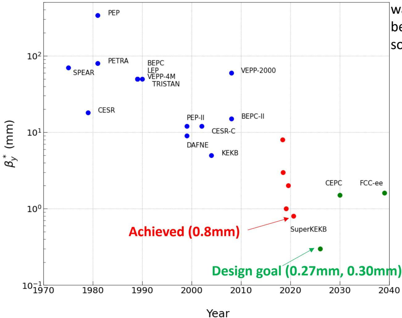
In 2022b run, we tried  $\beta_y^*=0.8\text{mm}$ . The specific luminosity was higher than  $\beta_y^*=1\text{mm}$  case. We could not store higher beam currents due to poor injection efficiency. We will re-try soon.
