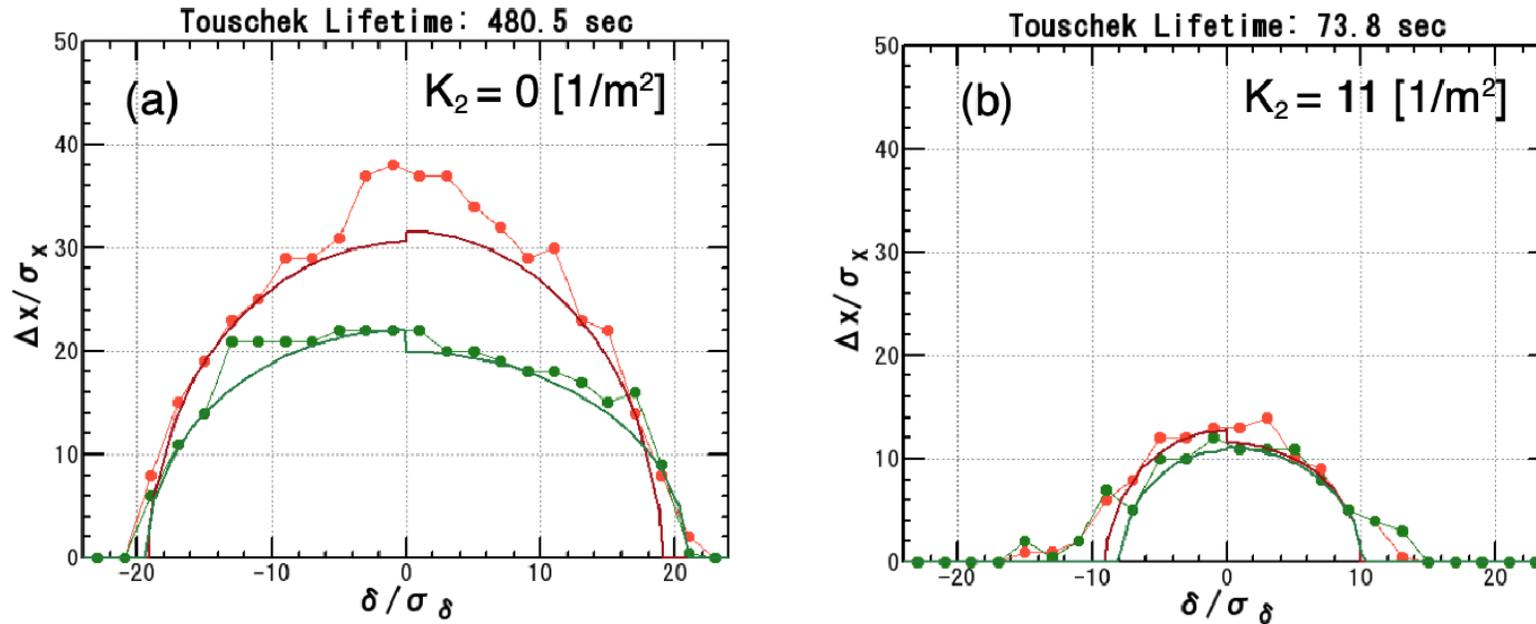
Figure 4.28: Dynamic aperture in the LER crab-waist lattice without beam-beam effect. Initial ratio of the vertical to the horizontal amplitude is 0.27 %. (a)  $K_2 = 0 [1/m^2]$ , (b)  $K_2 = 11 [1/m^2]$ .
