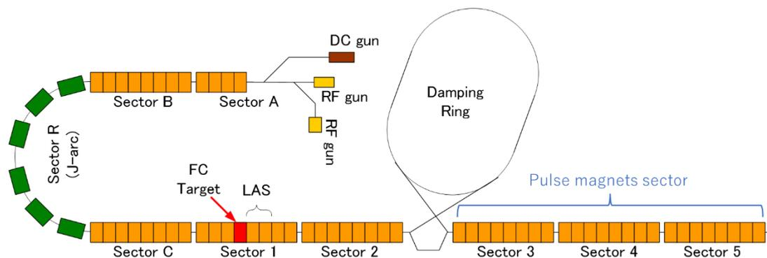
Figure 1: KEK injector linac.
