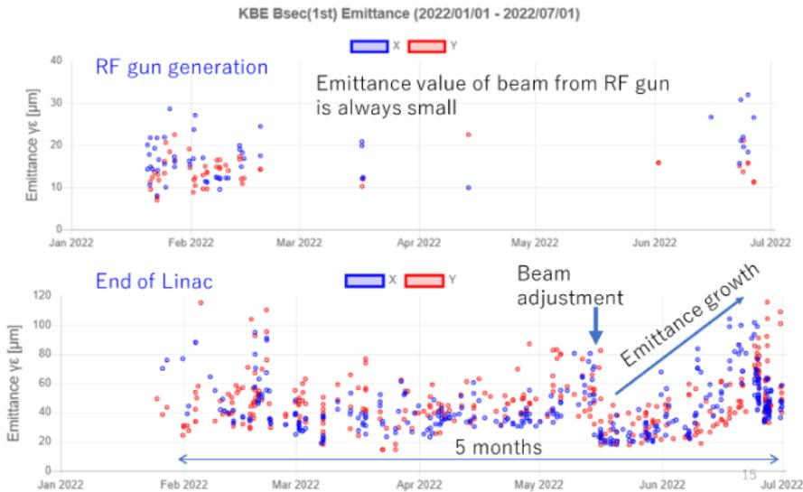
Figure 3: Long-term emittance value history of the electron beam. Emittance of RF gun beam (upper) and end of linac (lower).
