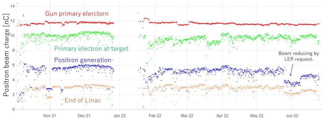
Figure 5: History of the positron beam charge for the LER.
