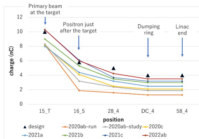
Figure 6: Long-term (a few years) charge history of the positron beam.
