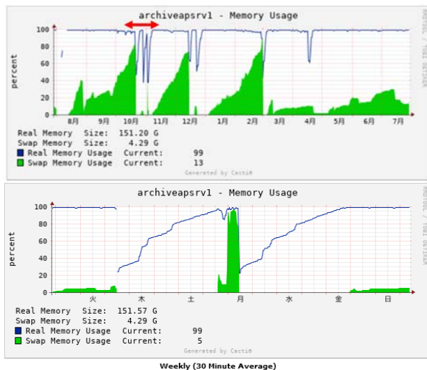
Figure 3: Screenshot of Cacti for memory usage on Archiver Appliance server in the recent past months (top) and around 2020.11.02 (top (red arrow term), bottom).
