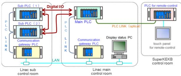
Figure 3: Schematic layout of safety management interlock system of Linac.
