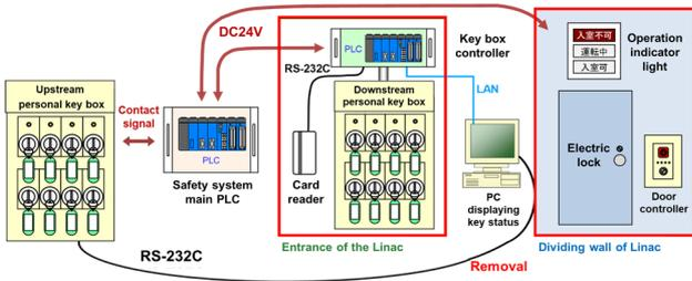
Figure 6: Schematic layout of the updated personal key management system to enter the accelerator room.
