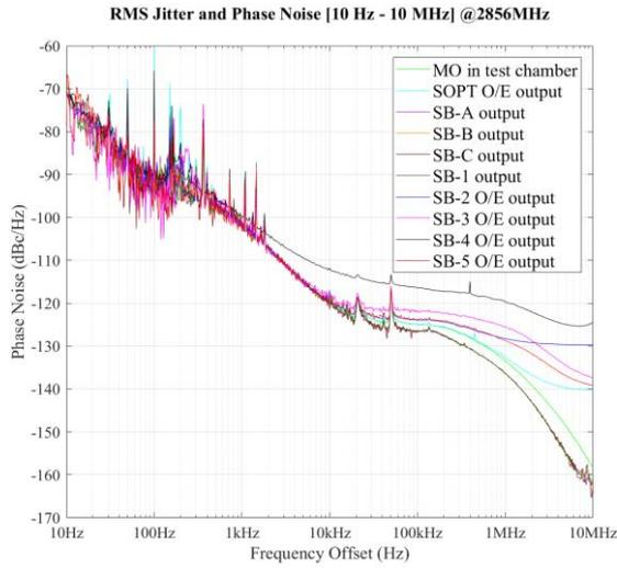
Figure 2: Single side-band phase-noise power spectrum of 2856 MHz REF of the optical links.
