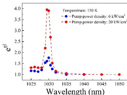
Figure 9: Gain test for different seed laser wavelength at 150 K under different pump power density.
