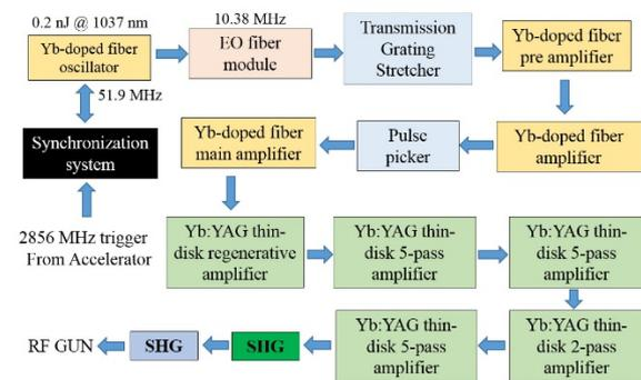
Figure 1: Layout of laser system.
