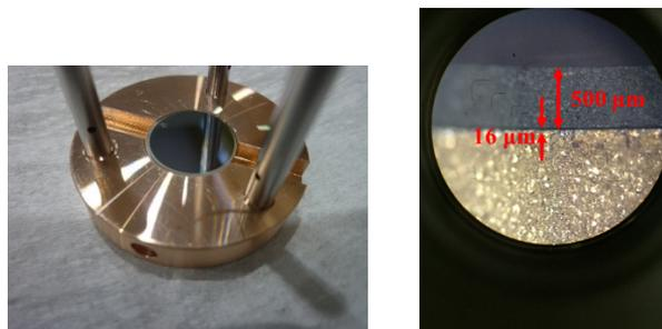
Figure 3: Accomplished Yb:YAG/Cu composite and side view under microscope.
