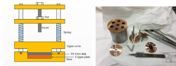
Figure 2: Configuration and components of fixtures for Au-Sn soldering.
