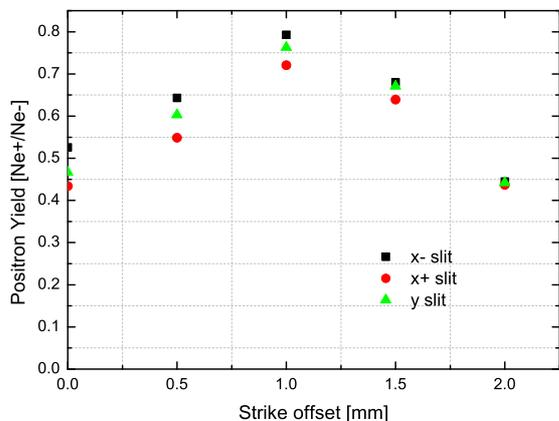
Figure 5: Positron yield as a function of electron bombardment position respect to the target center. Strike offset equals 0 is the target center and the primary electron beam's moving direction is toward to the central axis. The black, red and green marks represent the slit orientation of x-, x+ and y respectively, as marked in Fig.2
