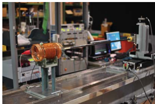
Figure 2: A straight slit FC made of OFC was set up on the experimental station.
