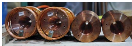
Figure 1: Four flux concentrator prototypes are manufactured and tested in KEK. From left to right: HRSC straight slit FC, OFC straight slit FC, OFC spiral slit FC and HRSC spiral slit FC.
