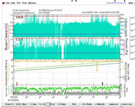
Figure 5: Typical one-day stored current variation of PF and KEKB rings during the simultaneous top-up operation.
