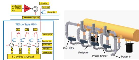
Figure 5: Tesla type linear PDS with a reflector and a phase-shifter in the downstream of the circulator.
