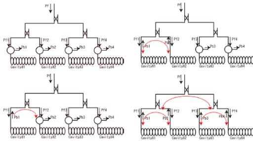
Figure 3: Procedure to eliminate the circulator in 3-dB hybrid PDS.
