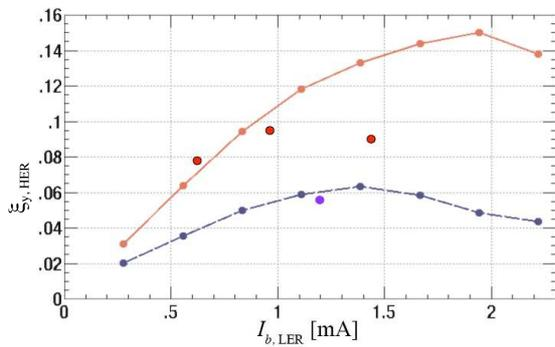
Figure 2: Predicted beam-beam parameters by the strong-strong beam-beam simulations with the crossing angle of 22mrad (purple) and the head-on (crab crossing) (red). Some experimental data are also shown with closed circles.
