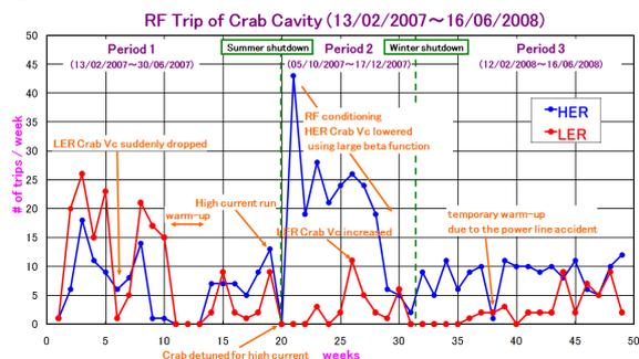
Figure 6: Trip rate of crab cavity system.
