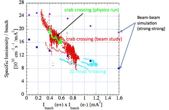
Figure 4: Beam current dependence of specific luminosity.
