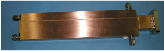
Figure 4: Photograph of a dummy load for C-band.
