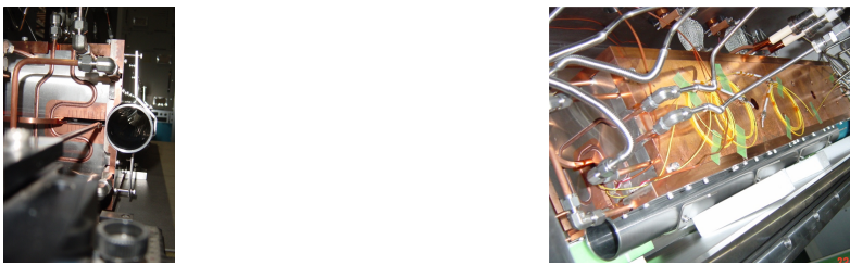
Figure 10.9: Photos of a prototype of the septum magnet. A mockup of the beam pipe made of ferromagnetic SUS430 stainless steel is attached on the septum conductor for the field measurement.
