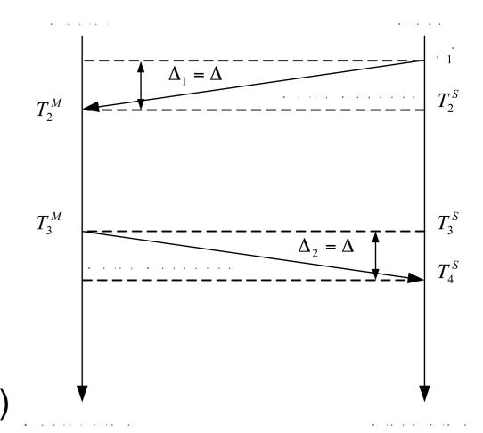
$$\Delta_{1} = T_{1}^{S} - T_{2}^{S} = T_{1}^{S} - (T_{2}^{M} + \delta)$$
