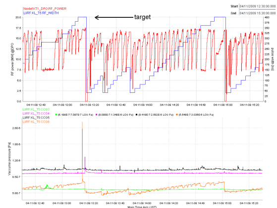
Figure 1: Typical example of variations in pulse width and RF power during processing.
