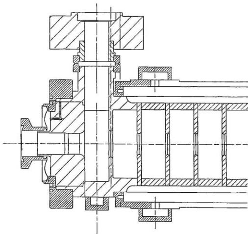
Figure 1: Input coupler of P5 section
