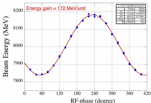
Figure 5: Energy gain measurement of C-band module
