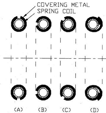
Figure 2: The cross-sectional forms of each seals
