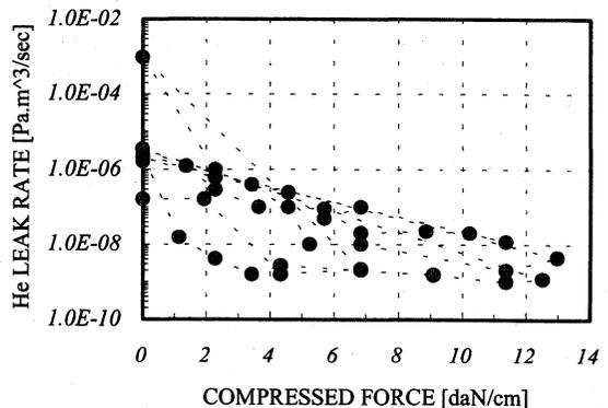
Figure 3: The compression power and a leak rate
