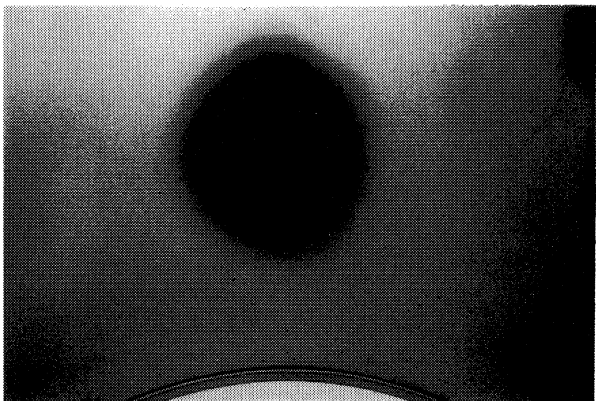
Fig. 1 Contamination of the Anode Ceramic.
