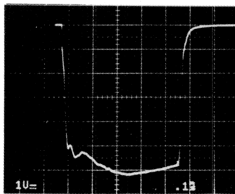
Fig. 4. Intensity versus time distribution of the total negative ion current extracted from a Cu sputter target at a voltage of -450 V and optimum cesium flow rate. Vertical axis: 1 mA/div. Horizontal axis: 0.1 msec/div.
