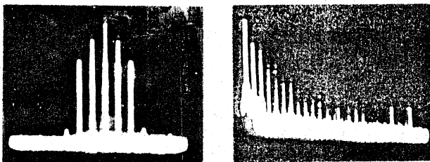
Figs. 5 (a), (b) The spectra of the RF noise (a, left), and of the beam signal (b, right). Spectrum lines appear at every 8 MHz.
