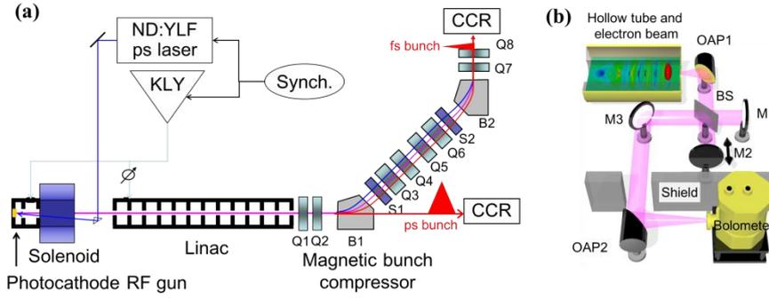
Figure 1: (a) Photocathode RF gun linac with a magnetic bunch compressor of an achromatic arc. (b) Diagram of multimode CCR and measurement system. OAP denotes an off-axis parabolic mirror; M, a plane mirror; BS, a beam splitter.
