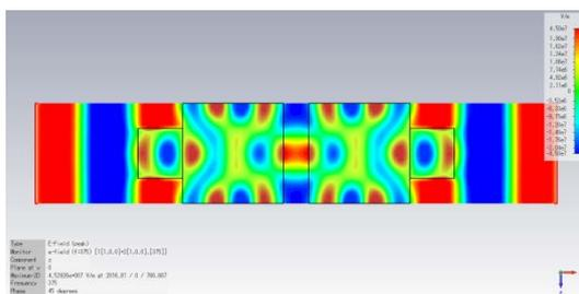
Figure 2. E-field (peak) z-component (accelerating field) distribution, colors represent the field strength and directions.
