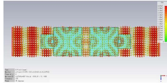
Figure 3. Arrow map of electric field distribution
