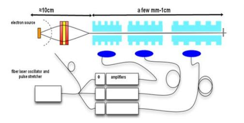
Figure 5. Schematic figure of multi-step acceleration.
