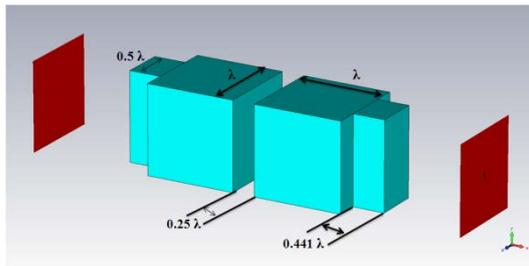
Figure 1. Dual grating structure dimensions.
